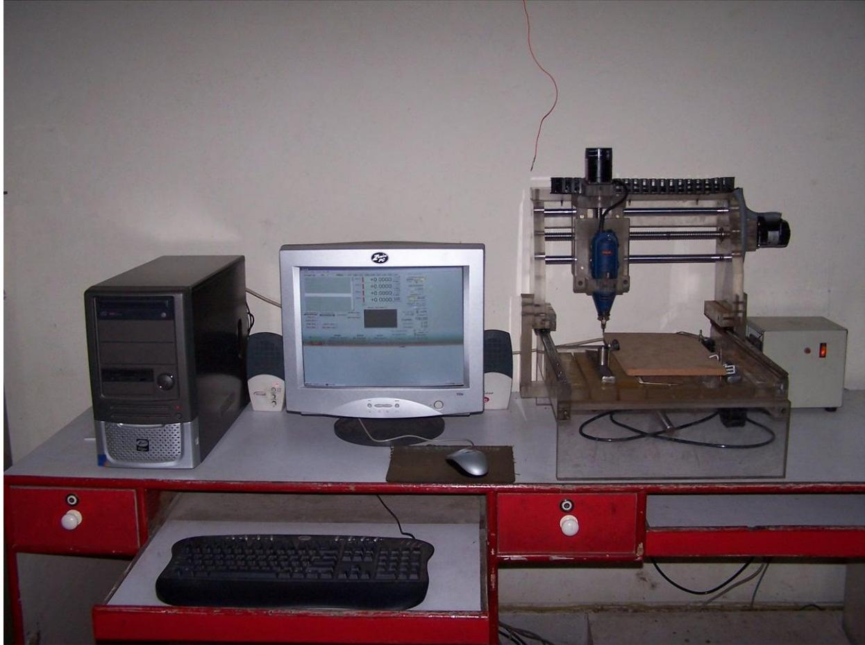
Here, User provides input in the Application which is being processed and then G-Code files are prepared by our System. These G-code files are fed as an input to an interface between CNC Controller and our application. CNC Controller now engraves the dimple and mark cuts into key using its blade. The position and all coordinates of CNC controller are defined in G-Code files.
